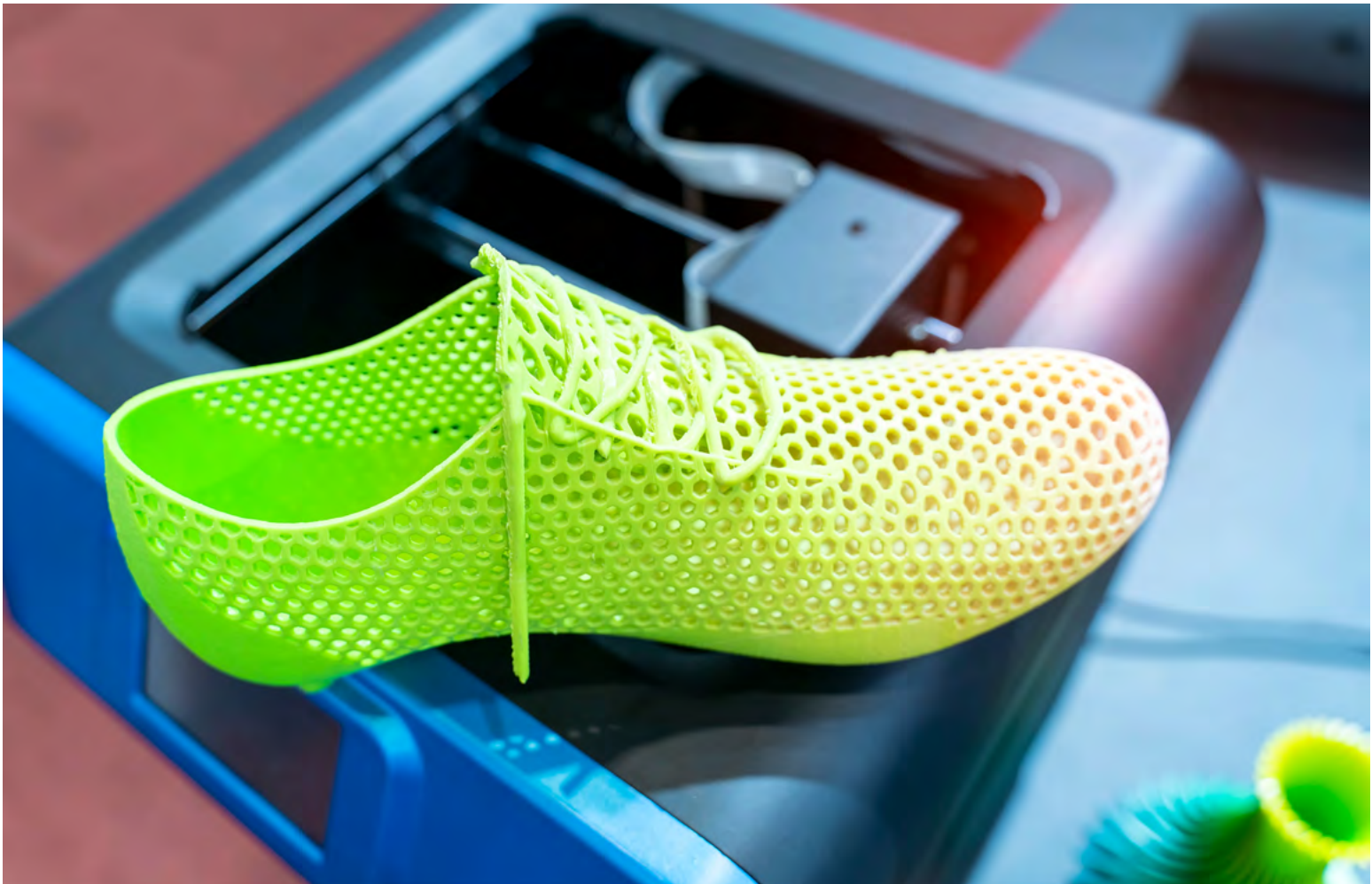
Companies like Superfeet already have 25 pilot stations around the United States to scan the soles of professional runners' feet and print custom shoes using 3D printers.
