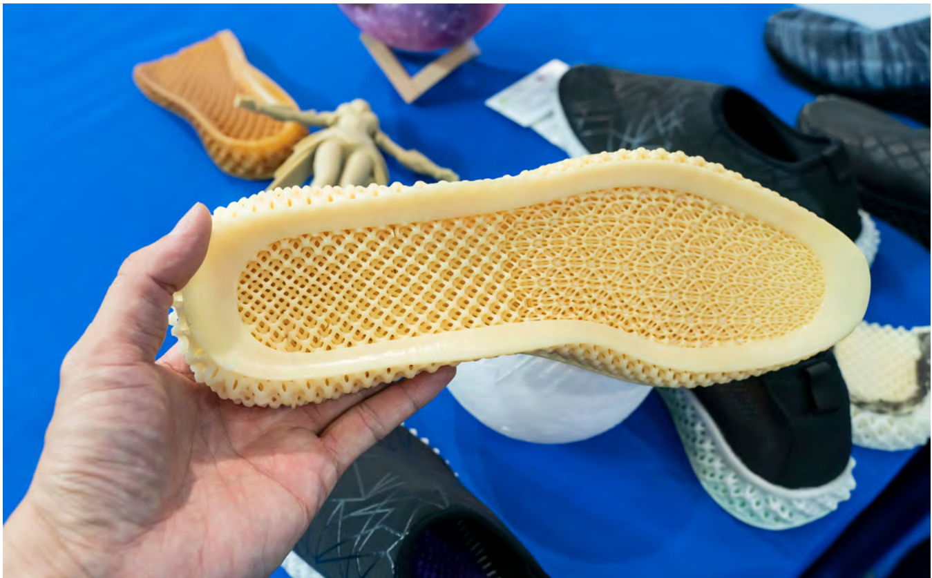
Companies like Superfeet already have 25 pilot stations around the United States to scan the soles of professional runners' feet and print custom shoes using 3D printers.
